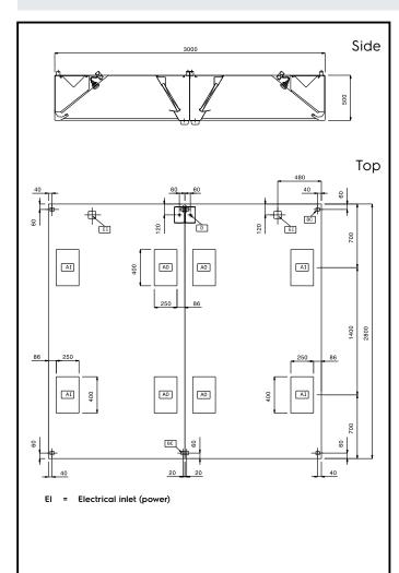
**Electric** Supply voltage: 641395 (STCF3028) 220 V/1N ph/50 Hz **Total Watts:** 0.48 kW Capacity: Supply capacity:  $0 \text{ m}^3/\text{h}$ **Key Information:** External dimensions, Width: 2800 mm External dimensions, Depth: 3000 mm 500 mm External dimensions, Height: Net weight: 364 kg
